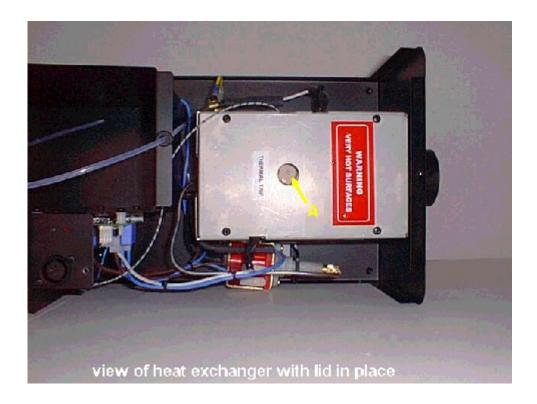
A. Hole in heat exchanger housing to access Thermal Trip
